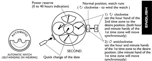
**Important:-** It is recommended to adjust the time by forwarding the hands instead of turning the hands backward. Please do not adjust the time during the period from 22:00 to 02:00, it could be harmful to the movement.
